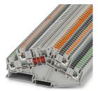
Disconnect terminal block, Current and voltage are determined by the plug used., Double level with angled contour, one disconnect knife, and one disconnect point, nom. voltage: 400 V, Thermal continuous current  $I_{th}$ : 16 A, 1st and 2nd level, connection method: Push-in connection, Rated cross section: 2.5 mm<sup>2</sup>, cross section: 0.14 mm<sup>2</sup> - 4 mm<sup>2</sup>, mounting: NS 35/7,5, NS 35/15, color: gray
