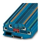
Disconnect terminal block, Current and voltage are determined by the plug used., nom. voltage: 400 V, Thermal continuous current  $I_{th}$ : 16 A, 1st and 2nd level, connection method: Push-in connection, Rated cross section: 2.5 mm<sup>2</sup>, cross section: 0.14 mm<sup>2</sup> - 4 mm<sup>2</sup>, mounting: NS 35/7,5, NS 35/15, color: blue
