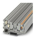
Disconnect terminal block, with test socket screws to accommodate 4 mm test plugs, nom. voltage: 500 V, nominal current: 20 A, connection method: Push-in connection, Rated cross section:  $4 \text{ mm}^2$ , cross section:  $0.2 \text{ mm}^2$  -  $6 \text{ mm}^2$ , connection method: Screw connection, Rated cross section:  $4 \text{ mm}^2$ , cross section:  $0.2 \text{ mm}^2$  -  $6 \text{ mm}^2$ , mounting: NS 35/7,5, NS 35/15, color: gray
