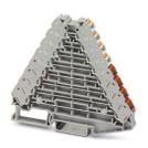
Marshalling panel, nom. voltage: 250 V, nominal current: 8 A, connection method: Push-in connection, 1st, 2nd, 3rd, 4th, 5th, 6th, 7th and 8th level, Rated cross section: 1.5 mm<sup>2</sup>, cross section: 0.14 mm<sup>2</sup> - 2.5 mm<sup>2</sup>, mounting: NS 35/7,5, NS 35/15, color: gray
