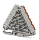
Marshalling panel, nom. voltage: 250 V, nominal current: 8 A, connection method: Push-in connection, 1st, 2nd, 3rd, 4th, 5th, 6th, 7th and 8th level, Rated cross section: 1.5 mm<sup>2</sup>, cross section: 0.14 mm<sup>2</sup> - 2.5 mm<sup>2</sup>, mounting: NS 35/7,5, NS 35/15, color: gray, color of connection elements: red
