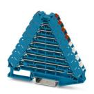
Potential distributors, without actuating push button, nom. voltage: 250 V, nominal current: 17.5 A, connection method: Push-in connection, 1st, 2nd, 3rd and 4th level, Rated cross section: 1.5 mm<sup>2</sup>, cross section: 0.14 mm<sup>2</sup> - 2.5 mm<sup>2</sup>, mounting: NS 35/7,5, NS 35/15, color: blue, color of connection elements: red, white
