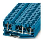
Feed-through terminal block, nom. voltage: 1000 V, nominal current: 76 A, number of connections: 3, connection method: Spring-cage connection, Rated cross section: 16 mm², cross section: 0.2 mm² - 25 mm², mounting type: NS 35/15, NS 35/7,5, color: blue
