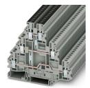
Multi-level terminal block, with equipotential bonder, nom. voltage: 500 V, nominal current: 19 A, connection method: Screw connection, Rated cross section:  $2.5 \text{ mm}^2$ , cross section:  $0.14 \text{ mm}^2$  -  $4 \text{ mm}^2$ , mounting type: NS 35/7,5, NS 35/15, color: gray
