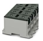
High-current terminal block, nom. voltage: 1000 V, nominal current: 380 A, number of connections: 2, number of positions: 1, connection method: Screw connection, Rated cross section: 240 mm<sup>2</sup>, cross section: 35 mm<sup>2</sup> - 240 mm<sup>2</sup>, Rated cross section: 240 mm<sup>2</sup>, cross section: 35 mm<sup>2</sup> - 240 mm<sup>2</sup>, mounting type: Screw mounting, color: black
