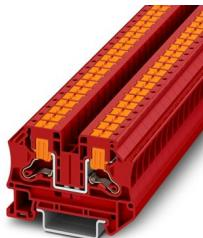
Feed-through terminal block, nom. voltage: 1000 V, nominal current: 41 A, number of connections: 2, number of positions: 1, connection method: Push-in connection, Rated cross section: 6 mm<sup>2</sup>, cross section: 0.5 mm<sup>2</sup> - 10 mm<sup>2</sup>, mounting type: NS 35/7,5, NS 35/15, color: red
