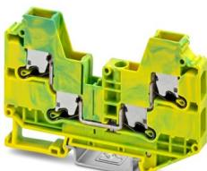
Ground terminal, number of connections: 4, number of positions: 1, connection method: Push-X-connection, Rated cross section: 6 mm<sup>2</sup>, cross section: 0.5 mm<sup>2</sup> - 10 mm<sup>2</sup>, mounting type: NS 35/7,5, NS 35/15, color: green-yellow
