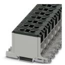
High-current terminal block, nom. voltage: 1000 V, nominal current: 145 A, number of connections: 2, number of positions: 1, connection method: Screw connection, Rated cross section: 50 mm<sup>2</sup>, cross section: 6 mm<sup>2</sup> - 50 mm<sup>2</sup>, Rated cross section: 50 mm<sup>2</sup>, cross section: 4 mm<sup>2</sup> - 50 mm<sup>2</sup>, mounting type: NS 35/15, NS 35/7,5, color: black
