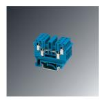
Feed-through terminal block, nom. voltage: 500 V, nominal current: 24 A, connection method: Screw connection, Rated cross section: 2.5 mm², cross section: 0.2 mm² - 4 mm², mounting type: NS 35/7,5, NS 35/15, NS 32, color: blue
