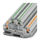
Double-level terminal block, nom. voltage: 1000 V, nominal current: 28 A, connection method: Push-in connection, 1st and 2nd level, Rated cross section:  $4 \text{ mm}^2$ , cross section:  $0.2 \text{ mm}^2$  -  $6 \text{ mm}^2$ , color: gray
