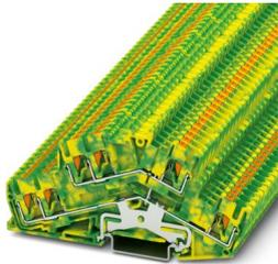
Double-level terminal block, number of connections: 6, connection method: Push-in connection, 1st and 2nd level, Rated cross section: 2.5 mm<sup>2</sup>, cross section: 0.14 mm<sup>2</sup> - 4 mm<sup>2</sup>, mounting type: NS 35/7,5, NS 35/15, color: green-yellow
