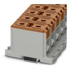
High-current terminal block, nom. voltage: 1000 V, nominal current: 220 A, number of connections: 2, number of positions: 1, connection method: Screw connection, Rated cross section: 95 mm<sup>2</sup>, cross section: 16 mm<sup>2</sup> - 95 mm<sup>2</sup>, Rated cross section: 95 mm<sup>2</sup>, cross section: 16 mm<sup>2</sup> - 95 mm<sup>2</sup>, mounting type: NS 35/15, NS 35/7,5, color: brown
