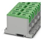
High-current terminal block, nom. voltage: 1000 V, nominal current: 290 A, number of connections: 2, number of positions: 1, connection method: Screw connection, Rated cross section: 150 mm<sup>2</sup>, cross section: 35 mm<sup>2</sup> - 150 mm<sup>2</sup>, Rated cross section: 150 mm<sup>2</sup>, cross section: 35 mm<sup>2</sup> - 150 mm<sup>2</sup>, mounting type: NS 35/15, NS 35/7,5, color: green
