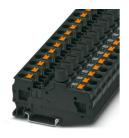
Fuse modular terminal block, fuse type: Glass / ceramics / ..., fuse type: G / 5 x 20, nom. voltage: 24 V, nominal current: 10 A, connection method: Push-in connection, Rated cross section: 6  $mm^2$ , cross section: 0.5  $mm^2$ - 10  $mm^2$ , mounting type: NS 35/7,5, NS 35/15, color: black
