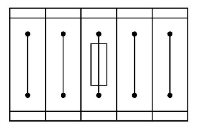
Fuse terminal block in single arrangement,
