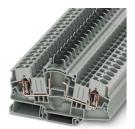
Component terminal block, If several diode terminal blocks need adding to the DIN rail, a spacer plate must be placed between them., with integrated P1000M diode, nom. voltage: 1000 V, nominal current: 5 A, connection method: Spring-cage connection, Rated cross section: 6 mm<sup>2</sup>, cross section: 0.2 mm<sup>2</sup> - 10 mm<sup>2</sup>, color: gray
