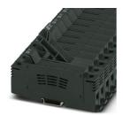
Fuse modular terminal block, fuse type: Glass / ceramics / ..., fuse type:  $gG / gPV / 10.3 \times 85$ , nom. voltage: 1500 V DC, nominal current: 32 A, number of positions: 1, connection method: Screw connection, Rated cross section: 16 mm<sup>2</sup>, cross section: 2.5 mm<sup>2</sup>- 25 mm<sup>2</sup>, mounting type: NS 35/7,5, NS 35/15, color: black
