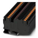
Fuse modular terminal block, fuse type: Blade, fuse type: C, nom. voltage: 48 V, nominal current: 25 A, connection method: Push-in connection, Rated cross section: 10 mm<sup>2</sup>, cross section: 0.5 mm<sup>2</sup>- 16 mm<sup>2</sup>, mounting type: NS 35/7,5, NS 35/15, color: black
