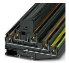
Fuse modular terminal block, fuse type: Glass / ceramics / ..., fuse type: G /  $5 \times 20$ , nom. voltage: 60 V, nominal current: 6.3 A, connection method: Push-in connection, Rated cross section:  $4 \text{ mm}^2$ , cross section:  $0.2 \text{ mm}^2$ - $6 \text{ mm}^2$ , connection method: Push-in connection, cross section:  $0.2 \text{ mm}^2$ - $6 \text{ mm}^2$ , mounting type: NS 35/7,5, NS 35/15, color: black
