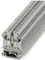
Feed-through terminal block, nom. voltage: 800 V, nominal current: 32 A, number of connections: 2, connection method: Screw connection, Rated cross section: 4 mm<sup>2</sup>, cross section: 0.2 mm<sup>2</sup> - 6 mm<sup>2</sup>, mounting type: NS 35/7,5, NS 35/15, NS 32, color: gray
