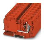
Feed-through terminal block, nom. voltage: 1000 V, nominal current: 125 A, number of connections: 2, connection method: Spring-cage connection, 1 level, Rated cross section: 35  $\text{mm}^2$ , cross section: 2.5  $\text{mm}^2$  - 35  $\text{mm}^2$ , mounting type: NS 35/7,5, NS 35/15, color: red
