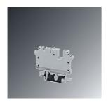
Double-level flange terminal block, for MSTB flange plug screw connection, nom. voltage: 250 V, nominal current: 24 A, number of connections: 3, number of positions: 1, 1 level, cross section: 0.2 mm² - 4 mm², mounting type: NS 35/7,5, NS 35/15, NS 32, color: gray
