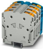
High-current terminal block, Blocked, nom. voltage: 1000 V, nominal current: 150 A, number of connections: 8, number of positions: 4, connection method: PowerTurn connection, 1 level, cross section: 10 mm<sup>2</sup> - 70 mm<sup>2</sup>, mounting type: NS 35/15, color: gray/blue
