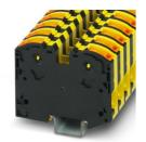
High-current terminal block, nom. voltage: 1000 V, nominal current: 125 A, number of connections: 2, number of positions: 1, connection method: PowerTurn connection, Rated cross section: 35 mm<sup>2</sup>, cross section: 2.5 mm<sup>2</sup> - 35 mm<sup>2</sup>, mounting type: NS 35/15, color: black/yellow
