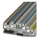
Installation ground terminal block, nom. voltage: 400 V, Thermal continuous current  $I_{th}$ : 22 A, Push-in connection, Rated cross section: 2.5 mm², cross section: 0.14 mm² - 4 mm², Push-in connection, Rated cross section: 2.5 mm², cross section: 0.14 mm² - 4 mm², mounting type: NS 35/7,5, NS 35/15, color: gray
