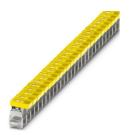
Connection terminal block, nom. voltage: 300 V, nominal current: 76 A, connection method: Screw connection, Rated cross section: 16 mm², cross section: 1.5 mm² - 16 mm², mounting: Neutral busbar, color: yellow
