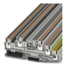
Installation ground terminal block, Current and voltage are determined by the plug used., nom. voltage: 400 V, nominal current: 22 A, Push-in connection, Rated cross section: 2.5 mm², cross section: 0.14 mm² - 4 mm², Push-in connection, Rated cross section: 2.5 mm², cross section: 0. 14 mm² - 4 mm², mounting type: NS 35/7,5, NS 35/15, color: gray
