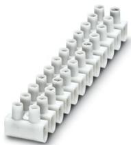
Polypropylene Europe terminal strip, white, for connecting solid conductors and stranded conductors with and without ferrules with a cross section of 1.5 to 16 mm<sup>2</sup>
