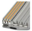
Feed-through terminal block, nom. voltage: 500 V, nominal current: 24 A, number of connections: 6, connection method: Push-in / plug connection, 1st, 2nd and 3rd level, Rated cross section: 2.5 mm², cross section: 0.14 mm² - 4 mm², mounting type: NS 35/7,5, NS 35/15, color: gray
