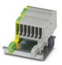
COMBI coupling, nom. voltage: 500 V, nominal current: 17.5 A, number of connections: 1, number of positions: 7, connection method: Push-in connection, 1 level, Rated cross section: 1.5  $mm^2$ , cross section: 0.14  $mm^2$  - 1.5  $mm^2$ , color: green/yellow-gray
