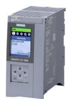
SIMATIC S7-1500F, CPU 1515F-2 PN, central processing unit with 1.5 MB work memory for program and 4.5 MB for data, 1st interface: PROFINET IRT with 2-port switch, 2nd interface: PROFINET RT, 6 ns bit performance, SIMATIC Memory Card required - - approvals and certificates according to entry 109817466 at support.industry.siemens.com to be considered! - -
