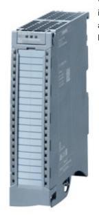
SIMATIC S7-1500 Analog output module AQ 4xU/I HF, 16 bit resolution, accuracy 0.1%, 4 channels in groups of 1; common mode voltage: 30 V AC/60 V DC, Diagnostics; Substitute value, isochronous mode; Delivery including infeed element, shield bracket and shield terminal: Front connector (screw terminals or push-in) to be ordered separately
