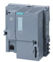
SIMATIC DP, CPU 1512SP F-1 PN for ET 200SP, central processing unit with work memory 600 KB for program and 2 MB for data, 1st interface: PROFINET IRT with 3-port switch, 25 ns bit performance, SIMATIC Memory Card required, BusAdapter required for port 1 and 2 \* \*\*\* approvals and certificates according to entry 109817615 at support.industry.siemens.com to be observed! \*\*\*\*
