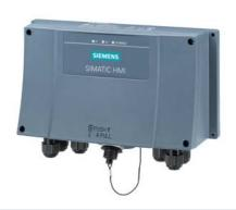
SIMATIC HMI connection box Standard for Mobile Panels, wall mounting, PROFINET and PROFIsafe, connection of safety relay, terminal detection, integrated switch
